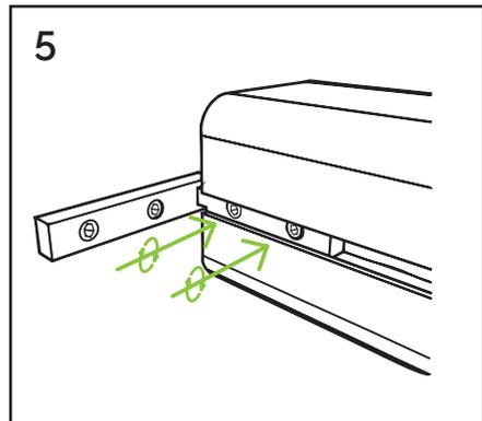
6. Slide Visirite side frame pieces keeping corner brackets within the channel.
