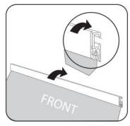
Press down firmly on top bar to secure graphic into place
