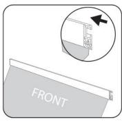
Place the plastic end caps back onto the top bar
