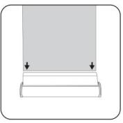
Peel the paper off the adhesive along the edge of the leader. Ensure the bottom of the banner is straight along thE adhesive ad attach the banner (front facing up)
