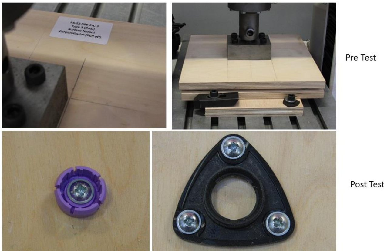
Figure 5.5 Type 3 Perpendicular pull test images
