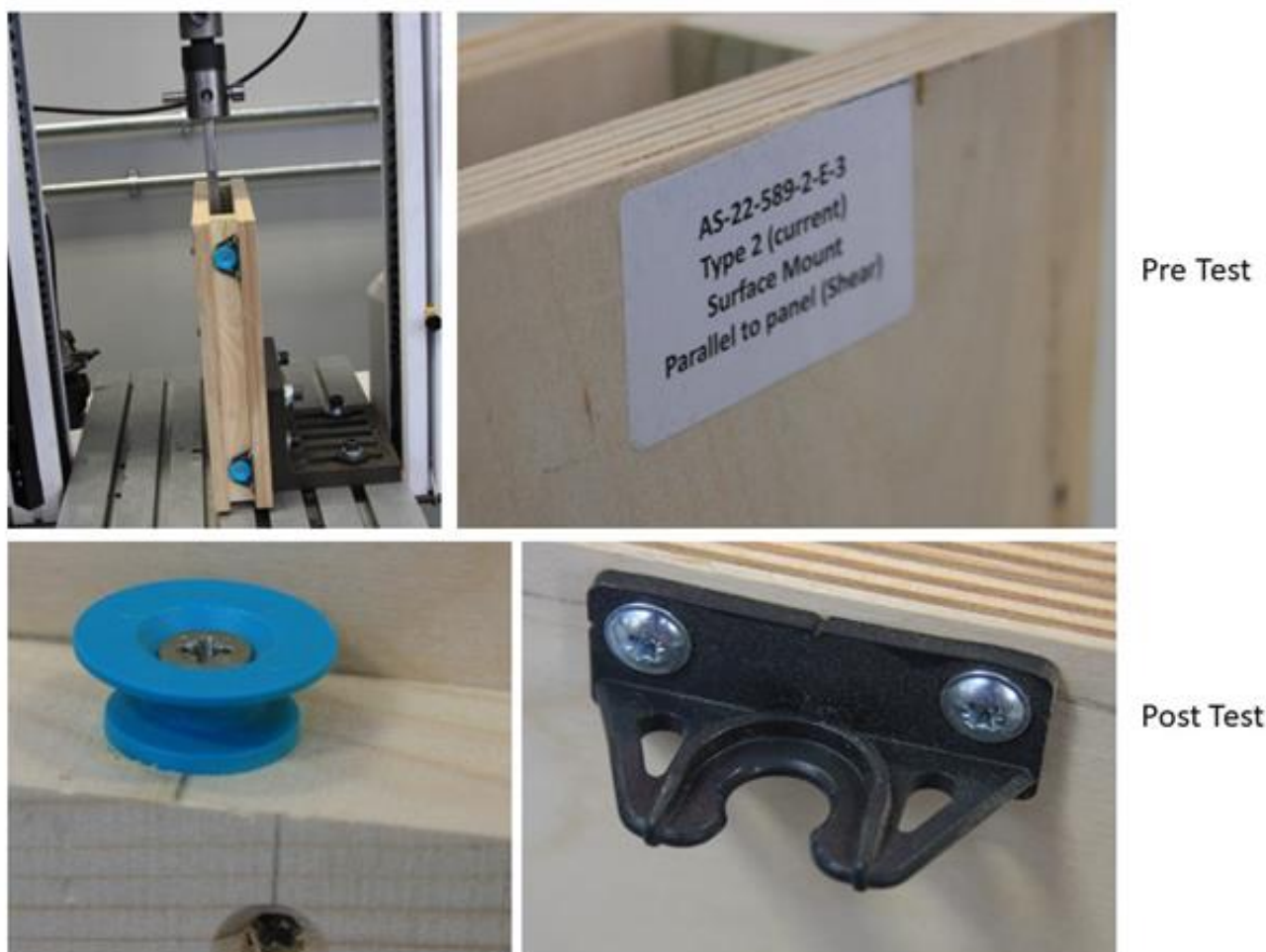
Figure 5.3 Type 2 Shear test images
