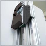
**Durable pneumatic cylinder enables swift, effortless movement of the cutting head, allowing for easy cutting of various materials.**
