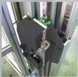
**Dual bearing blocks situated on a linear rail ensure dependable and precise guidance of the cutting head.**
