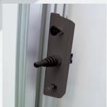
**The pneumatic clamping system provides a quick, effortless, and secure method for material handling, complemented by speed control for adjusting cutting velocity.**
